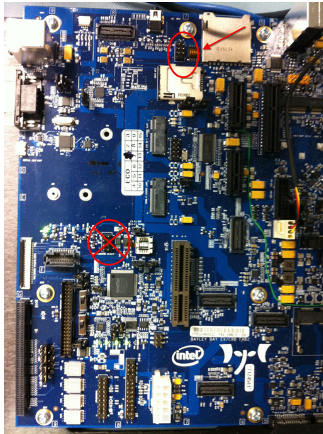
Figure 7. Programming Header Location Close-up
